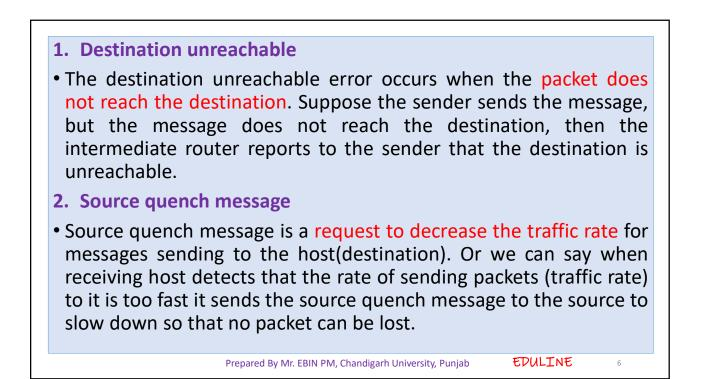
ICMP will take the source IP from the discarded packet and informs the source by sending a source quench message. Then source will reduce the speed of transmission so that router will be free from congestion.
